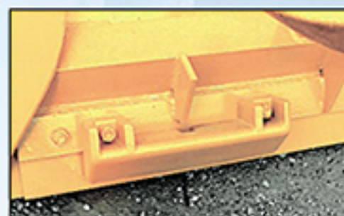
Moldboard Shoe For 6" or 8" cutting edges.
